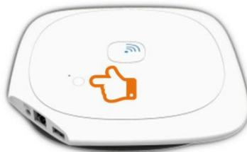
3. Wirelessly connect to the device using its default SSID. The default SSID is *Model Name\_xxxxxx* (Please see Figure 1 to find the Model Name), where “xxxxxx” is the last six digits of the Wi-Fi MAC address (WFM), which is printed on the bottom of the device. For example, for a device with a WFM of **F835DD85457A**, the wireless SSID is **WRTD-303N\_85457A**.
